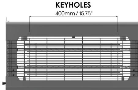
The unit simply hooks onto the 2 screws via the keyhole cut-outs in the rear of the unit. Drill 6mm holes to a depth of 35mm. Using the plastic plugs provided, insert the screws into the holes to leave 5mm protruding. Then hang the unit onto the 2 protruding screws ensuring it is secure.
