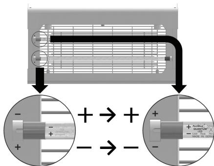
Replacing the LED tubes is the opposite procedure of removal.
