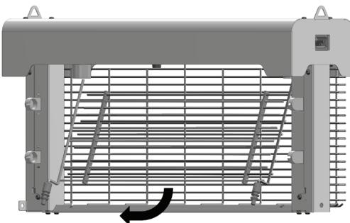
Re-assemble the unit in reverse order ensuring the grid is re-inserted into the spring-loaded connectors.
