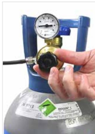
**(EN)** Open the valve on the CO<sub>2</sub> gas cylinder and adjust it to 0.5 kg per day by using the black knob.
