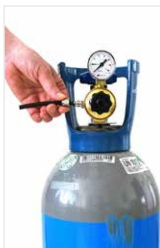
**(EN)** Use a wrench size 30 to fix the regulator on the gas bottle. Fix the free end of the CO<sub>2</sub> tube with the nut onto the outlet and re-screw the nut.
